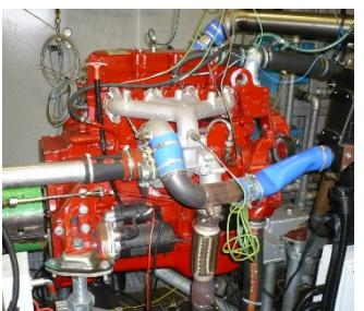
Gas diesel(dual fuel) engine – vehicle
