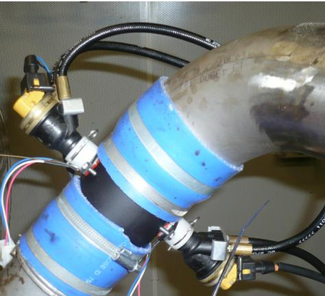
LPG Injectors are located between the intercooler and the intake manifold. The LPG supply is not synchronized with the suction stroke, the batch size is determined by the frequency and the opening time of the EV of the LPG injectors.
