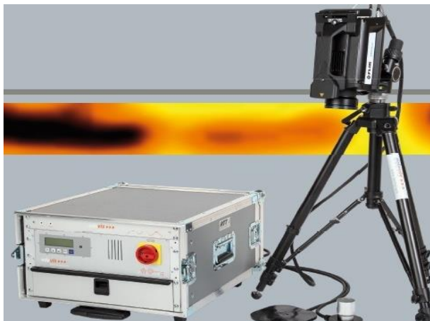
Measuring setup for the application of the active thermographic method for detecting weld defects
